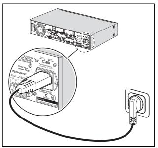
figure 3.2: Power connection and voltage selector
